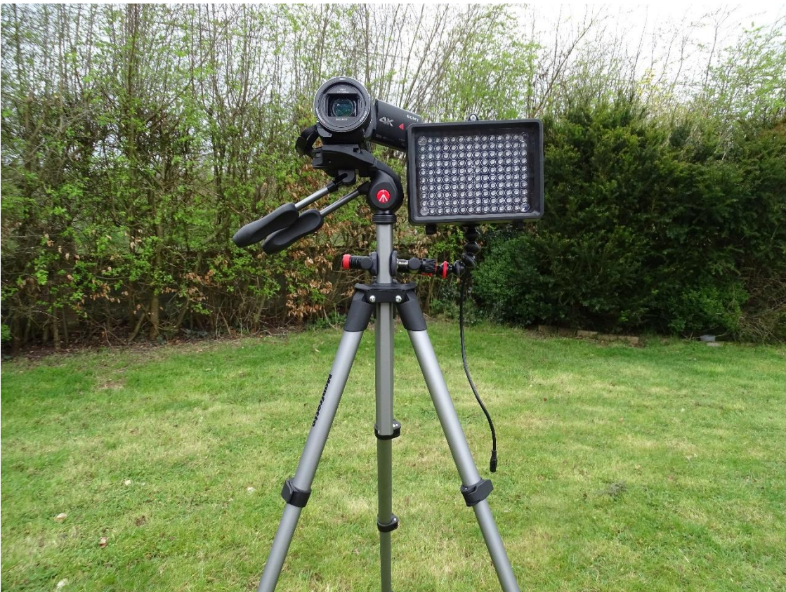
Plate A: These are demonstration photographs of the Thermal Imagery scope set up with Anabat Scout Full Spectrum bat detector and camcorder coupled with IR illuminator.
